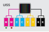
When the ink cartridge runs out of ink, the indicator will light up red, while the system already switches automatically to the second cartridge of the same color
