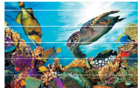
Gap / white streaks (Excessive paper feeding)
