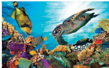
Overlap / black streaks (Insufficient paper feeding)
