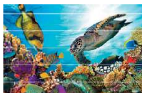
Gap / white streaks (Excessive paper feeding)
