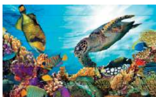
Overlap / black streaks (Insufficient paper feeding)
