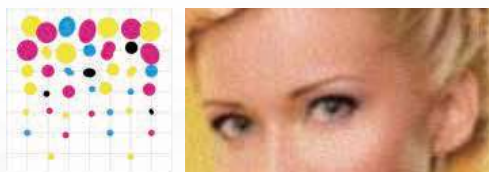
Gaps and overlaps occur between the dots, resulting in coarse image quality
