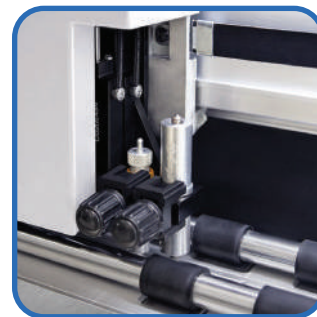
DOUBLE KNIFE HEAD DESIGN DIE-CUTTING & INDENTATION
